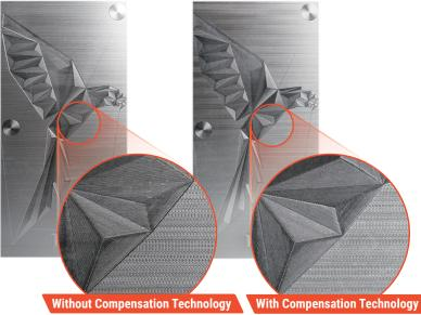
The edges between each areas are obvious before compensation. Whereas the edges on the workpiece after compensation are not obvious because the error is much smaller. The real cutting results shown with Takumi spindle thermal compensation, the thermal deformation is less than **5µm**.
