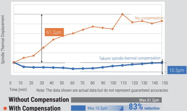
■ H10 with HEIDENHAIN TNC640; 15,000rpm direct drive; no machine warm up.
