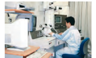
Using a transmission electron microscope to survey metal structure
