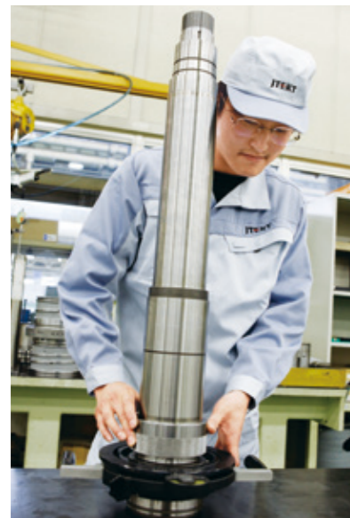
Dynamic balance measurement
