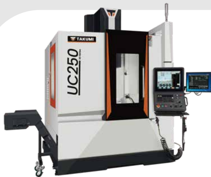
Takumi console operation panel with 15-inch touch screen and dual screen (optional).
