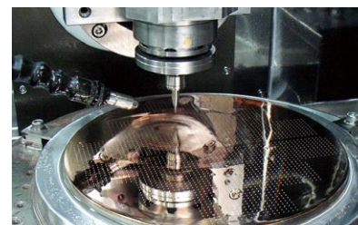
Machining wafer-level lens array mold
