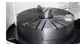
(28) Specification of hydraulic three-Jaws table
