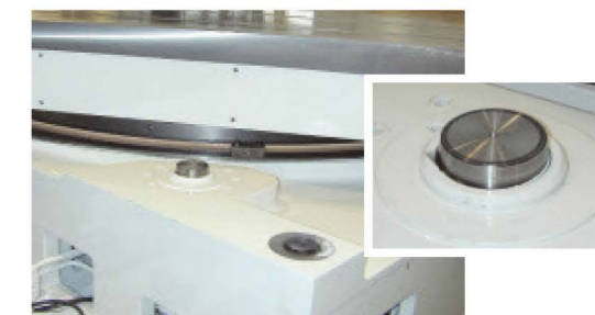
42 Rotary table locating pin at 90° locations
