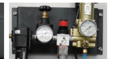
Air Limit(Workpiece contact surface check equipment)
