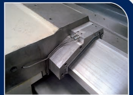
Double scrapers with compressed air for special guide ways security against grinding powder.
